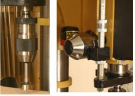
The keyless 5/8"-capacity chuck (left) and easy to use depth controls (right) make the PM2800 Drill Press versatile and easy to use.
